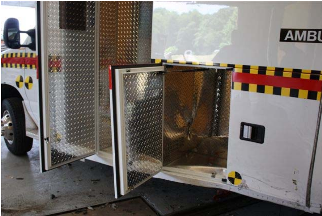
VIEW SHOWING DAMAGE TO INTERIOR OF LEFT SIDE STORAGE COMPARTMENT (TEST 055)
