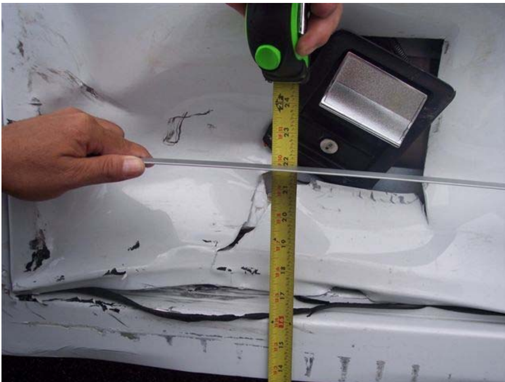
RIGHT SIDE IMPACT SHOWING MEASUREMENT OF MAXIMUM CRUSH (TEST #052)
