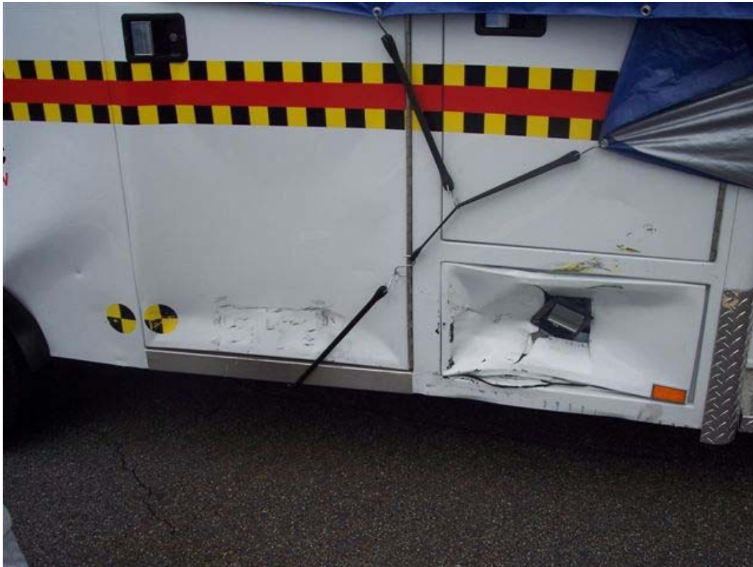
OVERALL VIEW OF RIGHT SIDE SHOWING DAMAGE TO PERSONNEL DOOR AND BATTERY COMPARTMENT (TEST 052)
