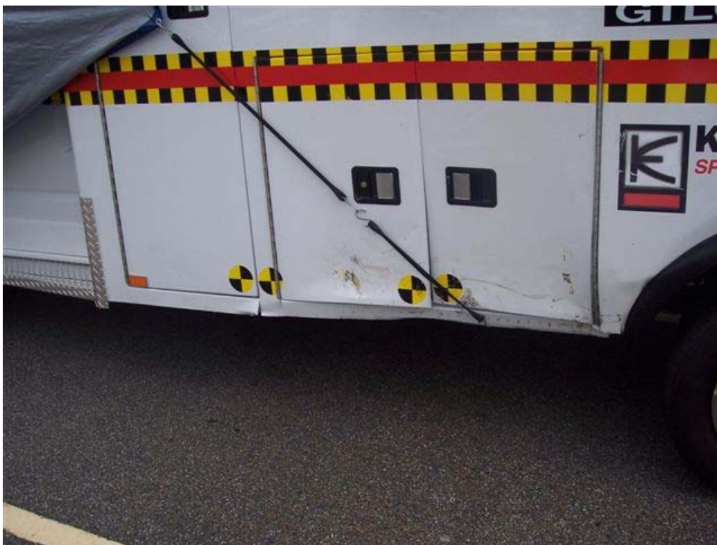
OVERALL VIEW OF LEFT SIDE DAMAGE (TEST #055)
